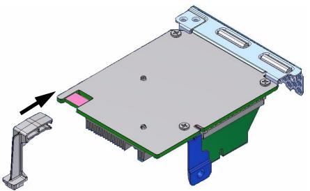
9. Push the Connector board into the card. The connector board must be installed as seen in Figure 9, directed toward the back of the server.
